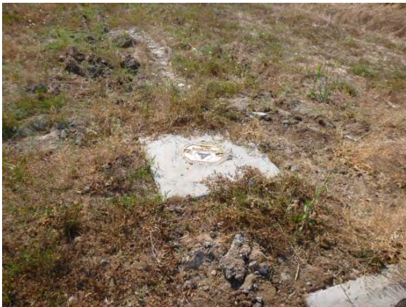
Photo 9: The site survey revealed a groundwater monitoring well next to the Huss Drive /Aztec Drive intersection.
